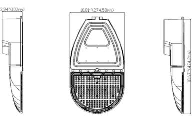
Unit: inch (mm) Shell materials: Aluminum & PC. Finish: Dark Bronze/White Net weight: 4.5Kg (9.9 lbs) Product Size: 474.2mm\*274.58mm\*100mm Carton Size: 536mm\*347mm\*170mm
